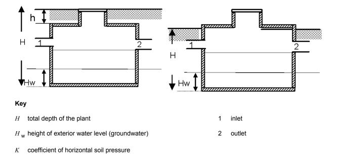
Figure 2 – Definition of parameters
